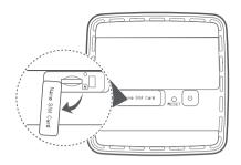
3 Insert the SIM card gently into the SIM card slot in the direction shown in the figure below until it clicks. Then close the SIM card cover.
